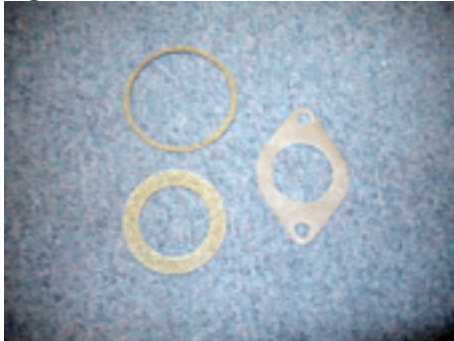
Figure 4 - The two round cork/rubber gaskets on the left were cut with the Olfa Compass Cutter and the paper gasket was cut with the hammer method.
