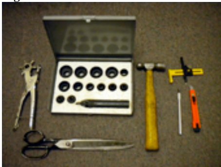
Figure 1 - Gasket making tools – hole punches and Olfa Compass Cutter (upper right) are essential for efficient, accurate cuts.
