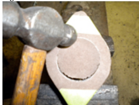
Figure 3 - A ball peen hammer is used to cut composition paper material for a simple cast metal piece (thermostat outlet).
