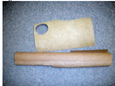
Figure 2 - Most gaskets can be made from various thicknesses of cork/rubber material (top) and composition paper in.
