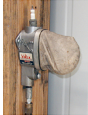
Figure 2, Basic spark plug cleaner; lever on side permits shifting from media to plain air.
